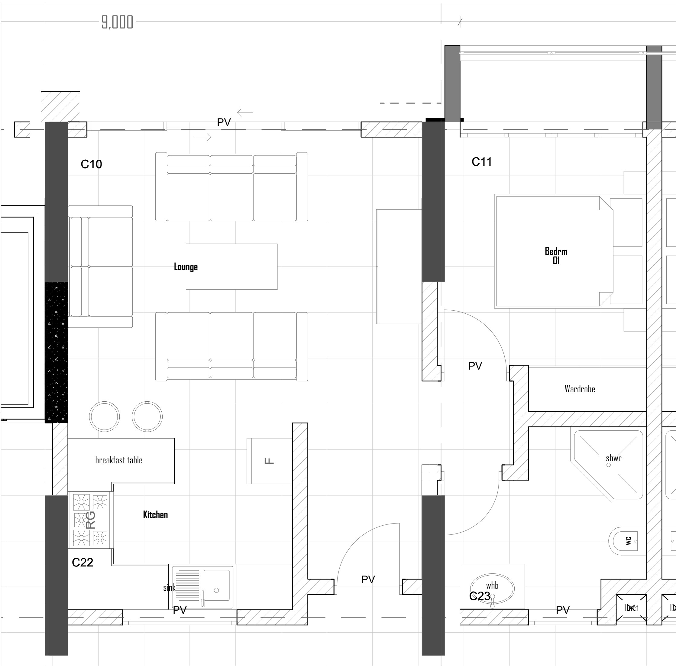
3. 1 BED TYPE A2 WITH BALCONY BLOWUP 1:30
